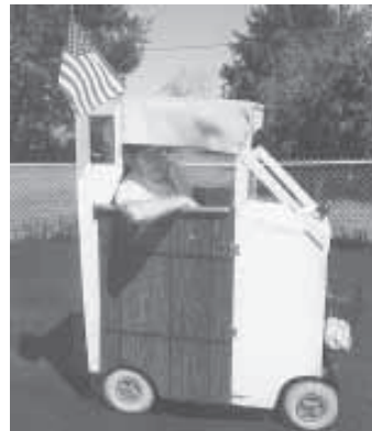
"Smokey" Stoll made a cab for his electric scooter that lets him drive comfortably around town no matter the weather. Cab has a hinged door on each side, a waterproof cloth top, and a plastic windshield and rear window.
