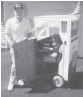
"Smokey" Stoll made a cab for his electric scooter that lets him drive comfortably around town no matter the weather. Cab has a hinged door on each side, a waterproof cloth top, and a plastic windshield and rear window.
