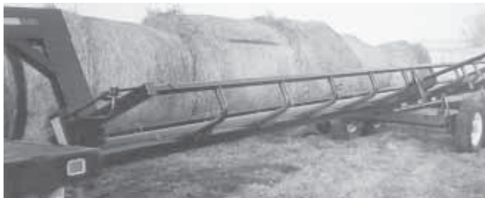
To unload bales, you pull back on a long lever that's attached to the cradle.
