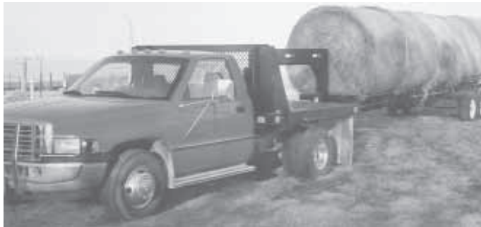
Tandem axle bale hauler is all mechanically-operated, with no hydraulics.
