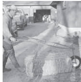
"Bale-Barrow" consists of two movable arms that attach to a single wheel. Arms are fitted with forks that grab onto bale.
