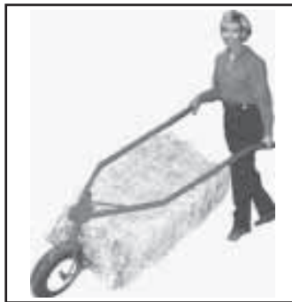
"Bale-Barrow" consists of two movable arms that attach to a single wheel. Arms are fitted with forks that grab onto bale.
