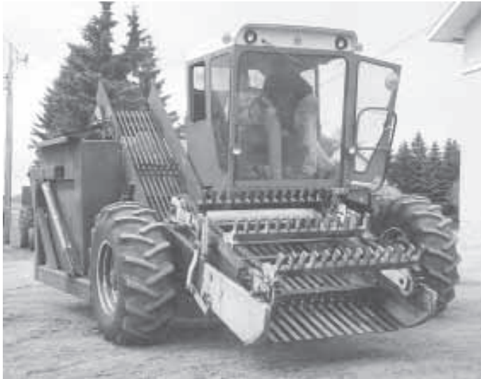
Based largely on parts from an old combine, Fairley's big rock picker has front drive wheels and a rear castor wheel that gives near instant response to changes in direction.
