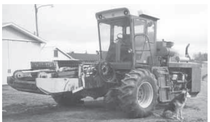
Cab mounts right behind rock-picking bed so Fairley has a clear view as he searches the field for rocks.
