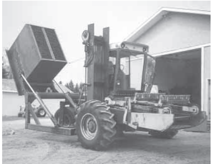
Rock conveyor swings up out of the way when box is dumped.
