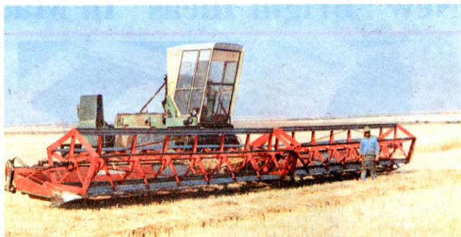
The two swather tables mount side-by-side on the 1977 Deere combine that Allemand bought for $2,500. A comparable commercial machine would have cost $75,000.
