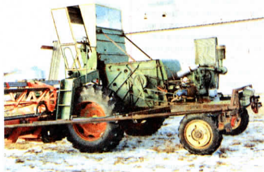
Allemand shortened the combine wheelbase 3 ft. and moved 303 cu. in. engine to the rear to counterbalance the swather tables.
