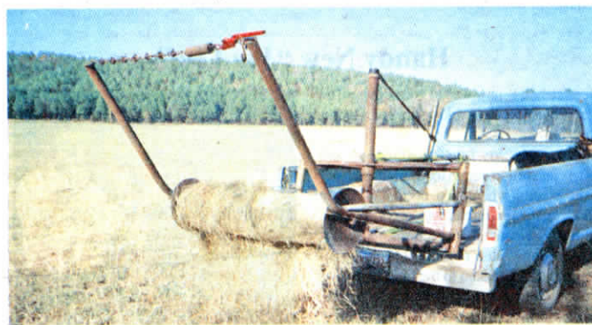
Old disc blades spin on 1-in. dia. pointed pins. A 2 1/2-in. dia. pipe acts as lifting mast.
