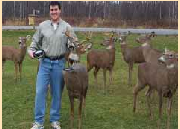
Life-like decoys are equipped with robotic heads and tails controlled by hand-held remotes. Head removes for transport.
