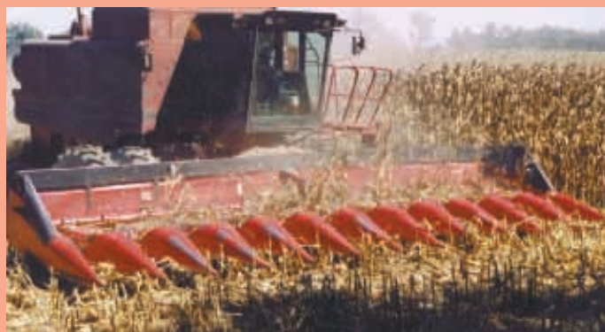
Gary Fesmire merged an 8-row header with a 4-row to build his own 12-row model.
