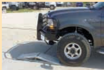
"Gogate" is activated by driving the left front tire of vehicle onto a metal ramp, or treadle.
