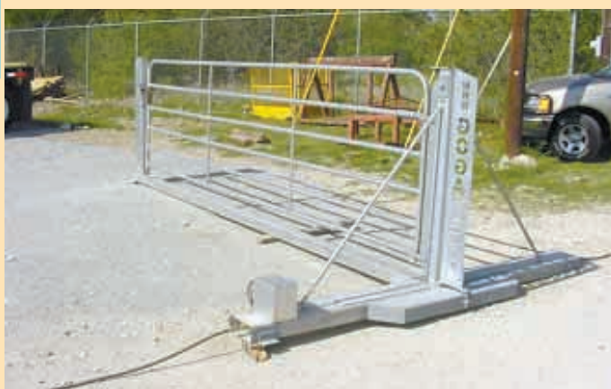
Treadle houses a cylinder filled with fluid. As treadle is compressed, the fluid activates a latch on the gate, allowing it to snap open.
