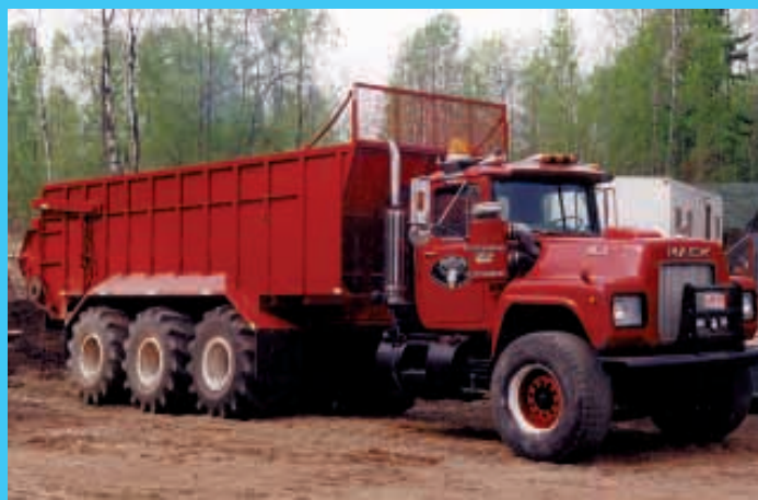
Gene Suteau converted a 1980 Mack tandem axle semi truck into this 6-WD, tri-axle model. It has a 24-ft. long, 9-ft. wide box that can haul up to 60,000 lbs. at a time.
