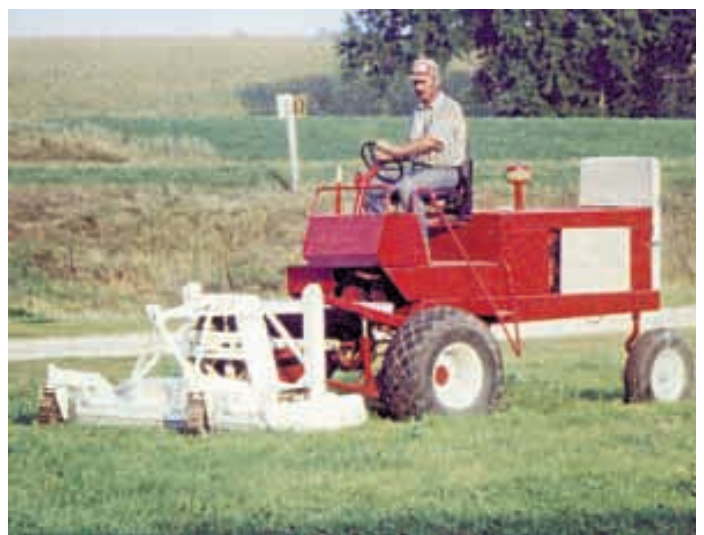
Arvin DeCook made this big zero-turn mower by mounting a pto-powered Woods mower on an old haybine.
