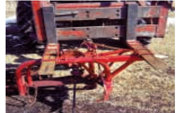
Mower slips onto loader forks and is belt-driven by an orbit motor.
