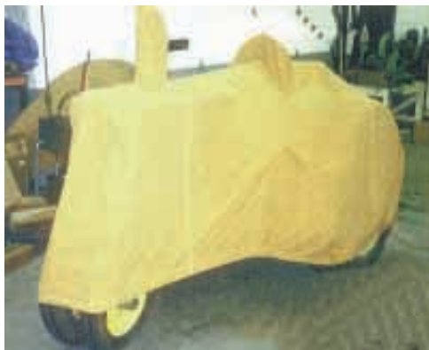
Soft flannel covers can be custom-fitted to tractors and wagons. Covers are made from water-resistant 12-oz. canvas on one side and soft flannel on the other.
