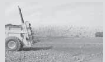
Joskin's "Tornado 2" is available in three different models with capacities ranging from 9 to 15 tons. Unit spreads manure in a pattern up to 40 ft. wide. An optional flail deck, consisting of twin spinners, can be installed on back, allowing you to spread lighter weight poultry manure in an extra wide pattern up to 60 ft. wide.
