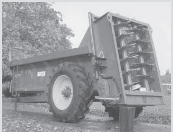
Bunning Lowlander comes in five different models with capacities ranging from 7 1/2 to 15 tons. Twin vertical beaters on back are equipped with high tensile cutting points.
