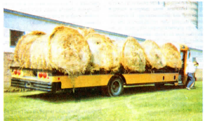
Luce cut off the top half of another bus, allowing him to haul 10 bales on the bottom layer and 13 or 14 on a second layer on top.
