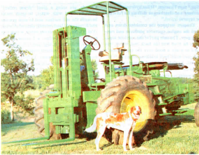
Laurence Stephens built this 8-ft. wide forklift out of an old Deere 55 combine.
