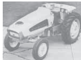
This IH HT-340 tractor was built in 1961 as part of a research project to develop a hydrostatic turbine-powered tractor.
