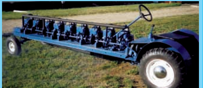
Engines belt-drive a jackshaft connected to a 4-speed transmission above rear axle.
