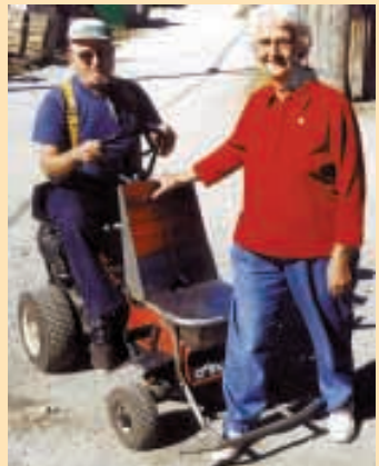
"It saves a lot of walking for both me and my wife," says Bob Lamb, who modified an 8 hp Ariens garden tractor by mounting a "shotgun" seat on the hood.
