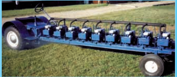
One-of-a-kind rig is powered by nine 5 hp Briggs & Stratton gas engines.
