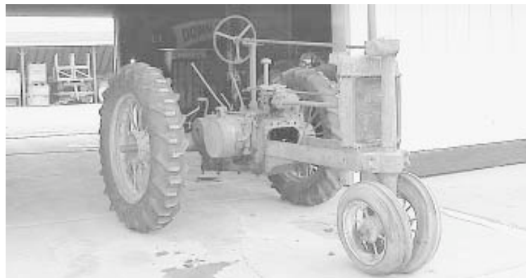
Photo shows a 1935 John Deere A before Spiegelberg Restoration started work on it for one of its customers. The job included having the crankshaft turned, the camshaft reground, the head overhauled, a new manifold installed, the carburetor rebuilt, and new magneto and main bearings.
