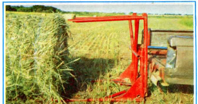
Forks slide down to ground over a roller at back end of pickup box.
