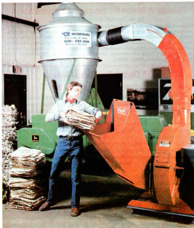
Photo shows Hundt feeding newspapers into modified wood chipper that blows shredded paper into "cyclone" above Deere square baler.
