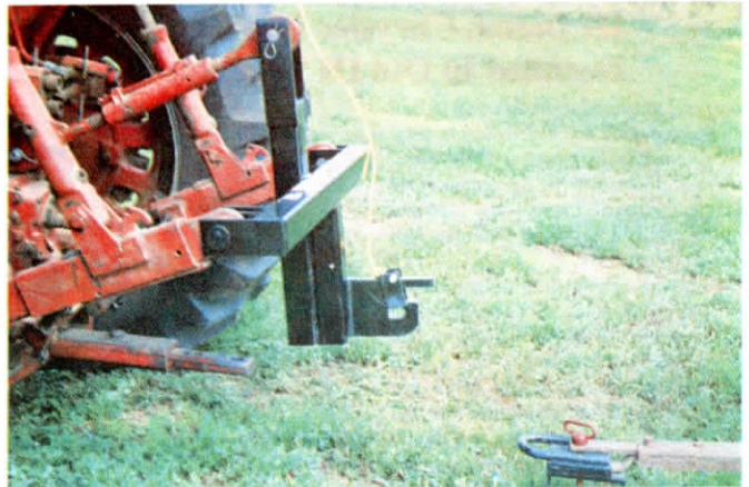
Catch loop slips over wagon tongue. Locking mechanism mounts on 3-pt. hitch.
