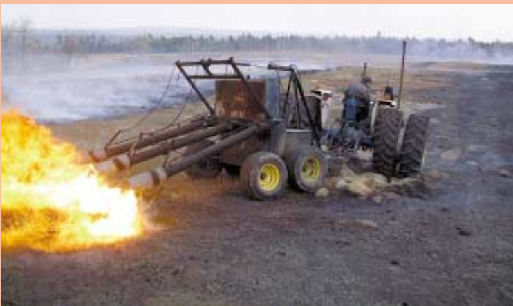
Tractor-mounted burner has three flame tubes protruding from back of machine.
