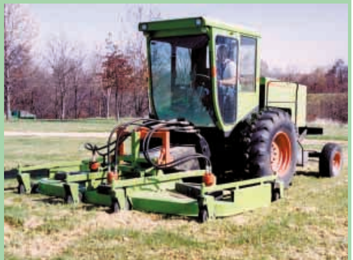
Bob Howard uses his home-built tractor for mowing, tilling and snowblowing. He built it mostly out of salvaged parts.
