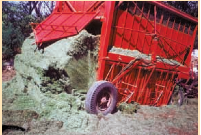
As the operator drives forward, the load is deposited on the ground and the pile automatically pushes the endgate open.
