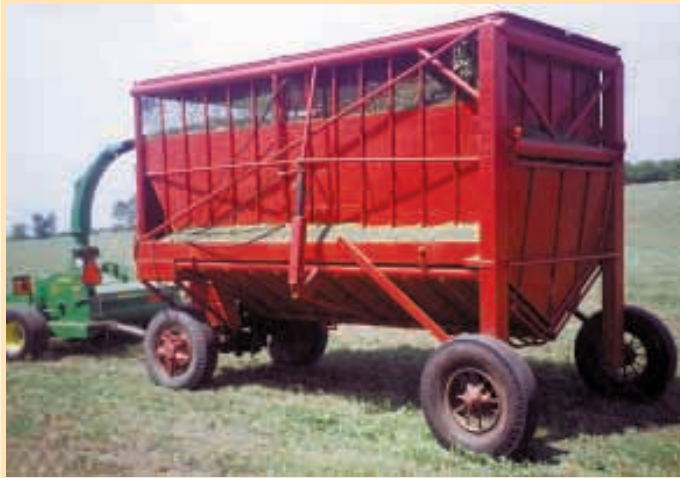
Home-built wagon has a hinged "trap door" on each side that slopes downward, and an endgate on back that's hinged at the top.
