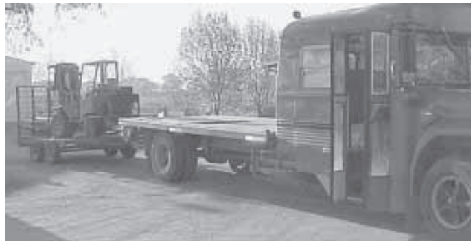
Jim Klassen converted an IH 65-passenger bus into a flatbed truck complete with a traveling office. He uses the "bus truck" during spring to deliver seed to farmers.
