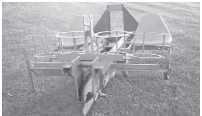
Tree planter is built on the main beam of an old pull-type plow. It's equipped with two plastic bucket boat seats and brackets to hold four 5-gal. plastic buckets.
