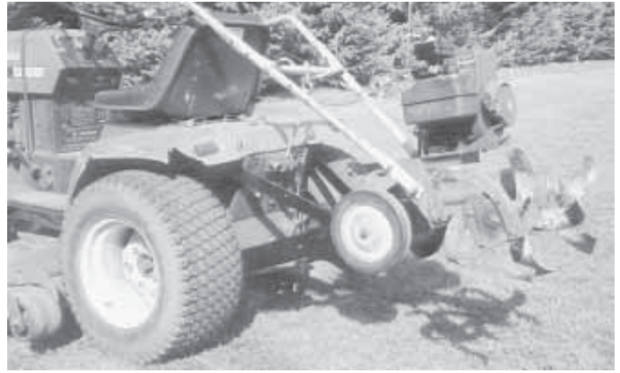
Leitzen 3-pt. mounted his walk-behind rototiller facing backward on his 16 hp Ariens garden tractor. To operate the rototiller he runs the tractor in reverse.
