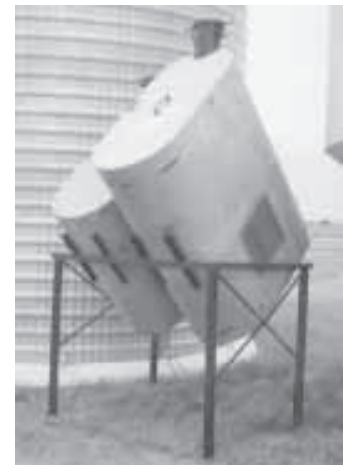
Brian Haubrich uses these metal spray tanks - set inside a four-legged metal stand at a 45 degree angle - to fill his grain drill.
