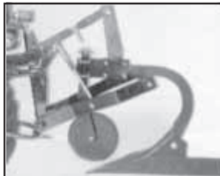
Rear hitch raises and lowers 10-in. moldboard plow.
