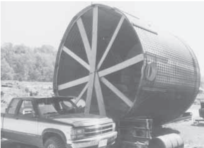
To keep the bottom of bin from collapsing under its own weight, the Wilson brothers criss-crossed the bottom opening with planks and tied them together at the center.
