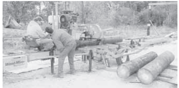
Sawmill owner Sharon Whitehurst specializes in turning treated posts into lumber. She uses a Wood-Mizer portable sawmill.
