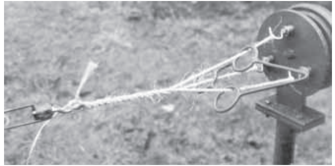
The drive wheel gear off an old reel-type lawn mower was used to make this rope machine. Guide rings are used to keep each strand of twine separate.
