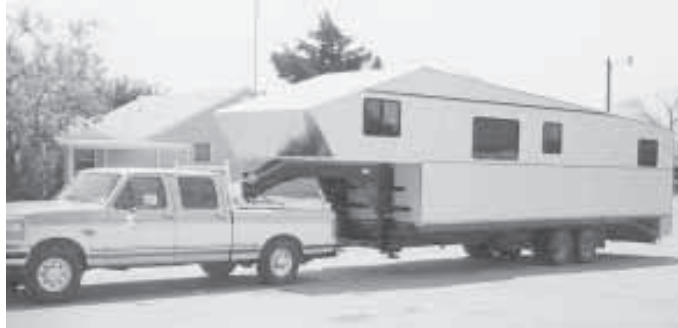
Camper attaches to gooseneck flatbed trailer with just four bolts.
