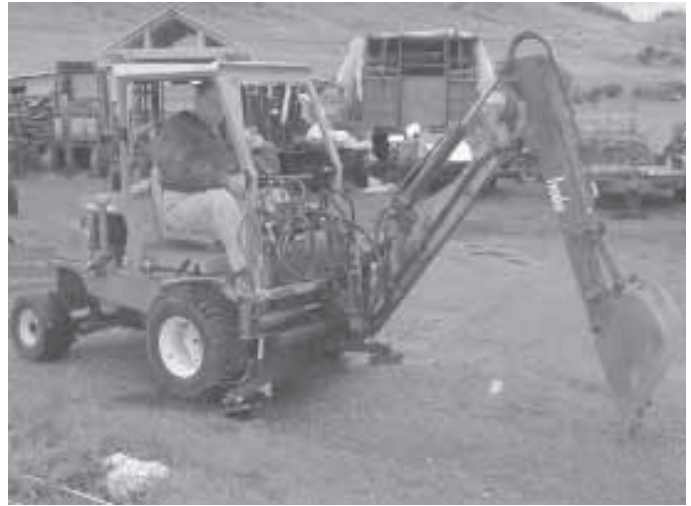
Ross Deal and his friend turned a Jacobsen riding mower into a self-propelled backhoe. "It can fit into areas where bigger commercial machines can't go," he says.
