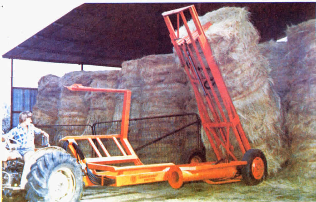
Crendon's Roll Chief picks up three bales at a time, stacks them on end, retrieves them from storage, and unrolls them for feeding.
