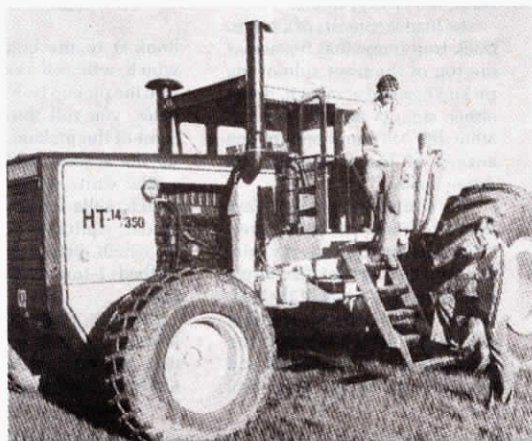
Ag Tech hauler is jointed in middle to break apart bales that have frozen together.
