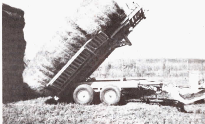
Ag Tech hauler is jointed in middle to break apart bales that have frozen together.
