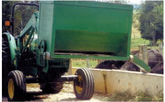
Ritter drives along his feedbunk to unload feed. A 12-volt electric motor belt-drives an auger that runs along bottom of hopper.
