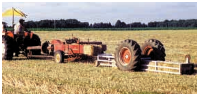
Zumberger put together a 16-ft. long frame to fit over the 14 by 18-in. bales from his New Holland baler. It's long enough to hold five bales.
