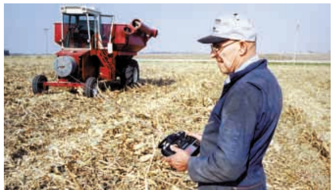
Louis Vaessen uses a model airplane controller to "drive" his self-propelled combine.
