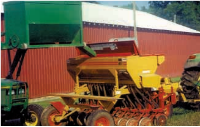
Powered hopper quick-taches to front-end loader and has a fold-down chute on one side. "Works great for loading seed into my grain drill," says inventor Greg Ritter.
