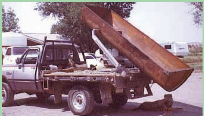
When bale spear lifts, tank slides backward and tips off the rear.
