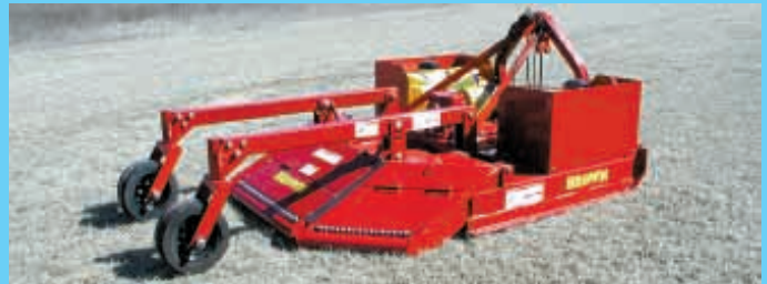
The 72-in. brush cutter deck cuts normally but has a brush roller on back that applies chemical to fresh-cut stubble.
