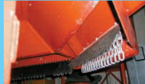
The 72-in. brush cutter deck cuts normally but has a brush roller on back that applies chemical to fresh-cut stubble.
