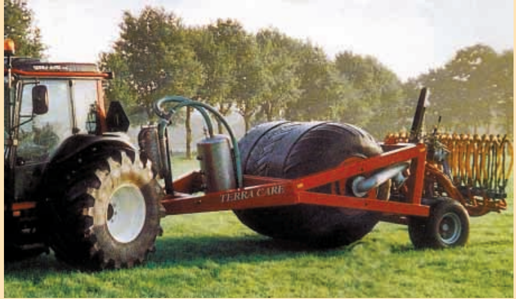
Sterken modified an 8-ft. wide, 6-ft. dia. flotation tire to carry a load of liquid manure. When full, it rolls on the ground.
