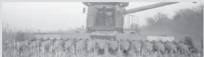
To make the 16-row head, Jensen cut a 4-row Deere head in half. Then he cut both ends off his 12-row head and added two rows from the 4-row head to each side..
