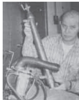
Metal plates in Spicer's hydrogen-maker are flooded with water, then charged electrically to split liquid into hydrogen and oxygen. He's used the system for more than 20 years.
