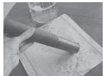
After item is removed from solution, it's "rust-proofed" for up to two weeks.
