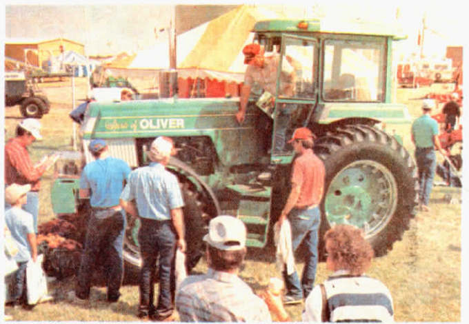
The "Spirit of Oliver" tractor is actually a modified White 185.
