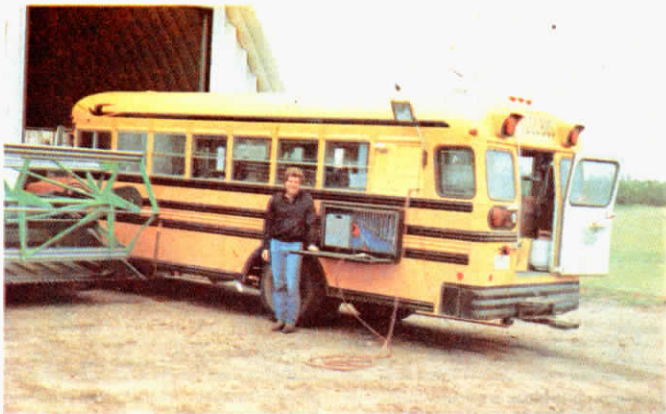
A drop-lid toolbox on the outside of the bus provides a convenient work station complete with air hose, water, electricity and a large lamp.
