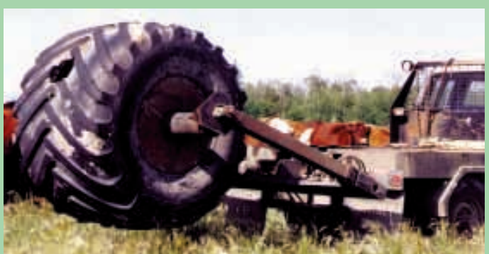
To raise and lower the tire, Belsheim uses the big round bale handler mounted on back of his 1-ton pickup.
