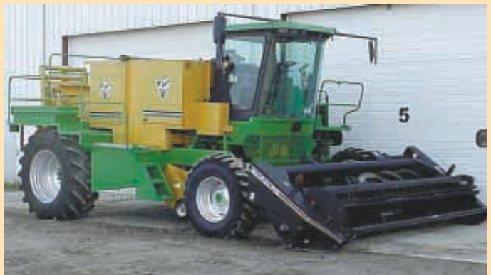
Gary Kelderman put together this direct-cut baler that cuts and bales in one pass.
