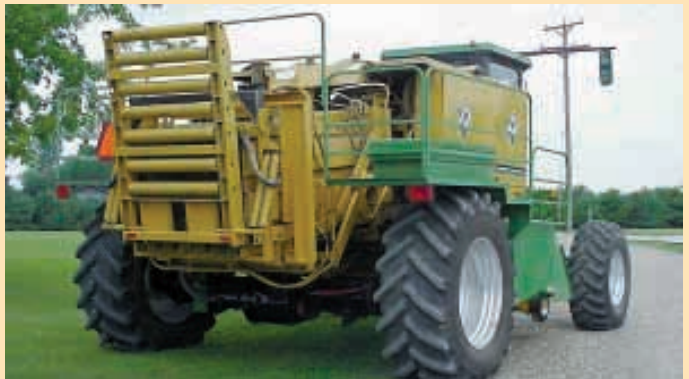
A Freeman big square baler and a Deere cab mount on a Kelderman factory-built frame. A 14-ft. sickle head up front cuts the dried grass and feeds it to the baler.
