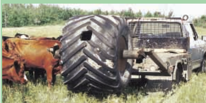
Pellets fall out of 7-in. sq. hole cut into the tread of 4-ft. wide floater tire. Tire drops a pile of pellets every revolution, spaced about 15 ft. apart.
