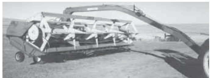
"It works great and I saved a lot of money over the cost of a new machine," says Edwin Egli, who mounted a 21-ft. Deere grain head on a Hesston 1014 hydroswing swather.
