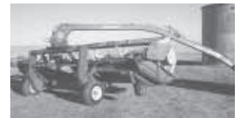
To keep the Deere grain head from interfering with the Hesston's swing pole, Egli raised the pole by adding 30 in. to its base.
