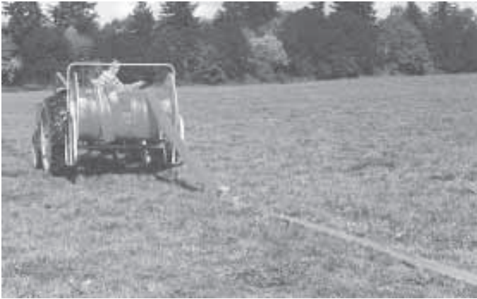
Baars Irrigation System consists of 1,000 ft. of flexible 3 by 4-in. hose on a 3-pt. reel.
