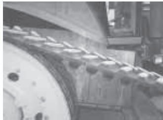
Plywood shield goes under top of belt and down 45 degrees from fender toward axle. It catches most of the residue and deflects it down, away from tractor frame.
