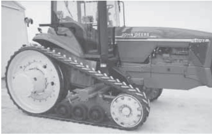
Jason Brown made his own shields to keep crop residue from building up near the muffler on his Deere 8410T tracked tractor.
