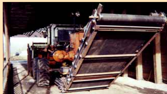
Rear conveyor lifts compost 10 ft. in the air before dropping it back on the pile.
