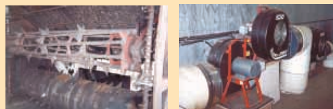
A 10-ft. long, 2-ft. dia. rotating drum with teeth pulls compost onto the conveyor belt.
