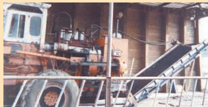
Modified snowblower on front pulls compost onto conveyor that runs under tractor to another conveyor on back.
