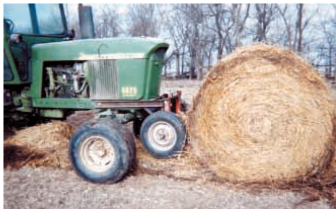
Bob Willats built his own low-cost bale unroller by mounting a pair of 14-in. wheels on spindles that bolt to the front of his Deere 4020 tractor.
