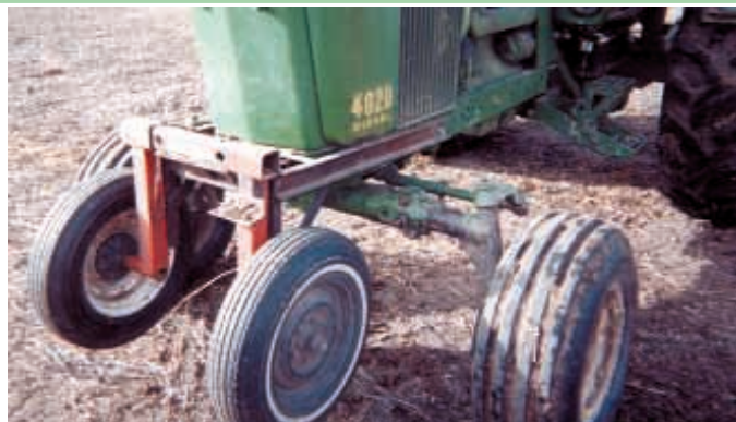
The wheels, spaced 2 ft. apart and about 1 ft. off the ground, spin freely.
