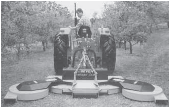
“Variable 360” mower uses a pair of hydraulic cylinders to open or close the wings.
