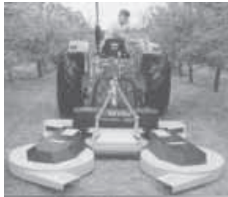
Mower can be narrowed down to a width of 6 ft. 8 in. from its maximum width of 12 ft.
