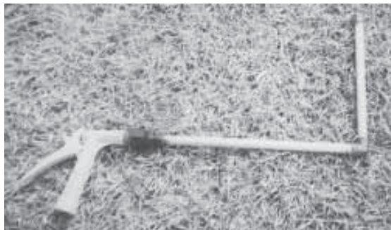
Clark’s “pistol grip” rinser consists of a water hose pistol with two lengths of aluminum pipe attached to it in the shape of an “L”. A brass nozzle mounts at end of pipe.
