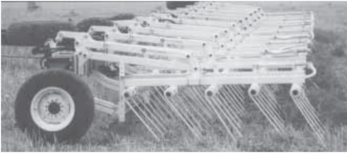
"It lets you mow stubble and work the residue all in one pass," says Coombs Mfg. about its new harrow. It's equipped with a flexible floating cutterbar on front.
