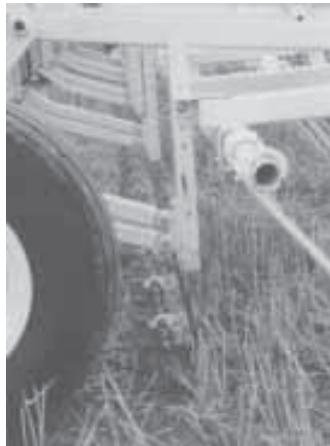
Flexible floating cutterbar mounts on parallel linkage to follow ground contour. Harrow controls cutterbar working height.
