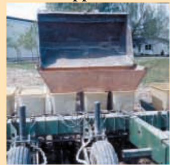
Plywood hopper fits over three row units at a time. It has one large opening on top that matches the bucket on his skid loader.
