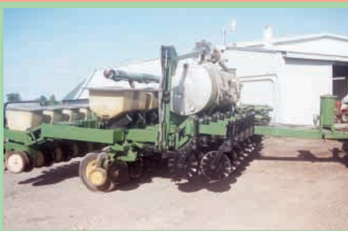
Friedrich built this 10-row, 21 1/2-in. planter. Front bar carries a 650-gal. liquid N tank and an independent hydraulic-controlled coulters toolbar with 3 coulters per row.
