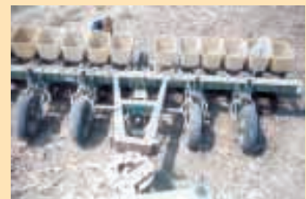
Scott Marbach and his father converted a used Deere 7000 12-row, pull-type corn planter into this 12-row, 16-in. narrow row soybean planter.
