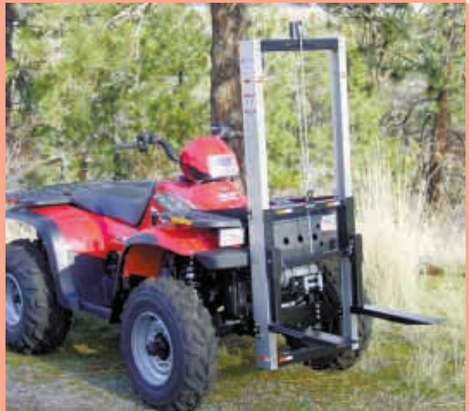
Newest product for 4-wheelers is this forklift that can safely lift and haul up to 200 lbs. Lifting height is 36 in. - high enough to place items in the bed of a full-size pickup.
