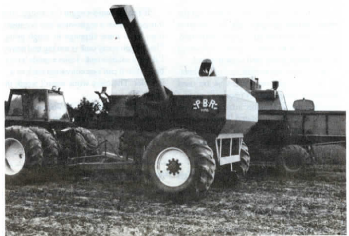
The cart holds 370 bu. To get that capacity the hopper is positioned ahead of the axle indicator at the front of the hopper tells the driver whether the auger cover is open or closed.
