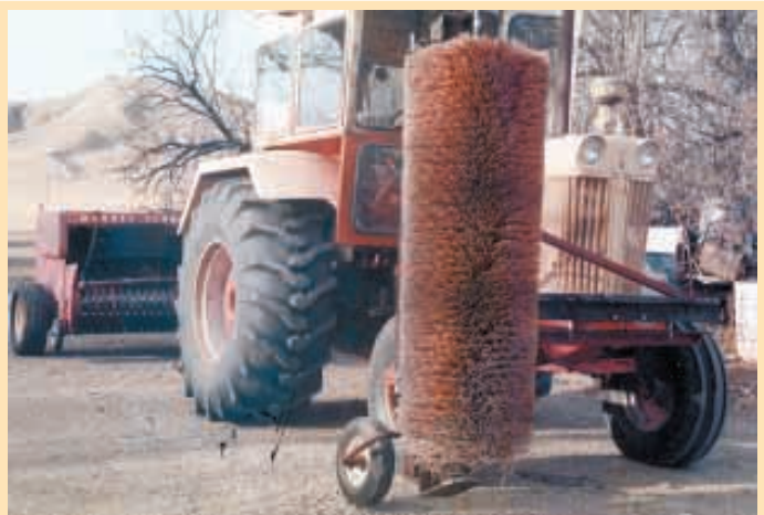
Frank Mayo mounted a 5-ft. high, 2-ft. dia. plastic "street brush" on front of his Case tractor. "I use it on CRP ground to sweep weeds off fence lines. It throws them into a windrow and I bale them up - all at the same time," he says.
