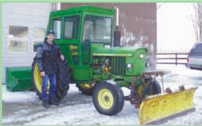
Robert Wuytenburg couldn't find a used cab for his Deere 2120 tractor. So he modified the cab off a Case 1031 diesel tractor and painted it green.
