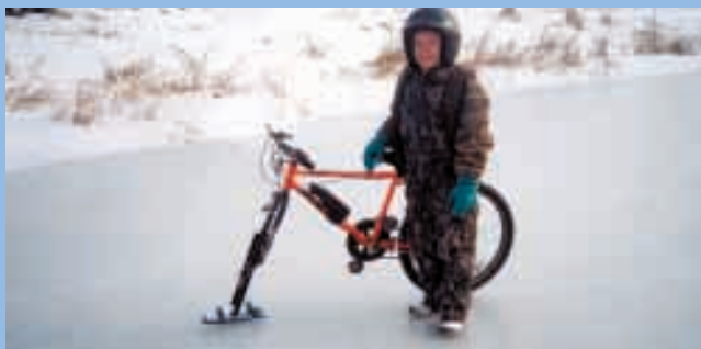
"It's amazing how well it works," says Harold Fratzke, who modified his grandson's 10-speed bike so he can ride it on frozen ponds and lakes.
