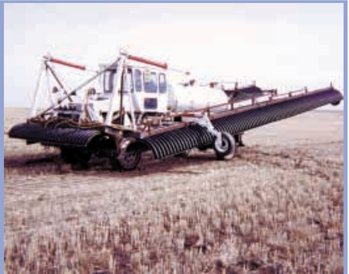
Sprayer's three-section folding boom is covered by a windshield made from corrugated plastic tile.
