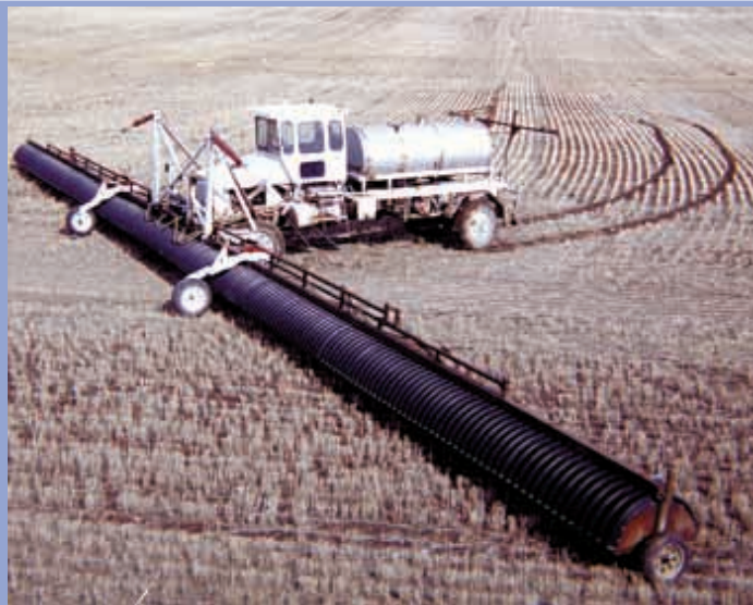
Sprayer is equipped with a 90-ft. boom with flexible tubing along it for two separate spraying systems.
