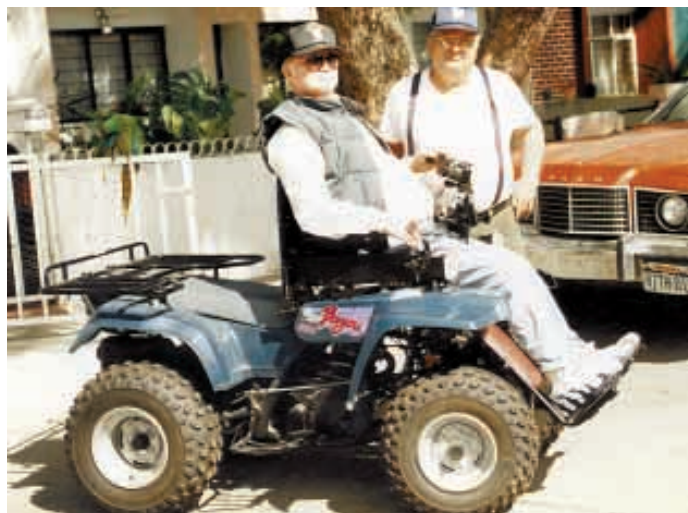
Wheelchair bolts onto front part of ATV frame. Driver has easy access to controls.
