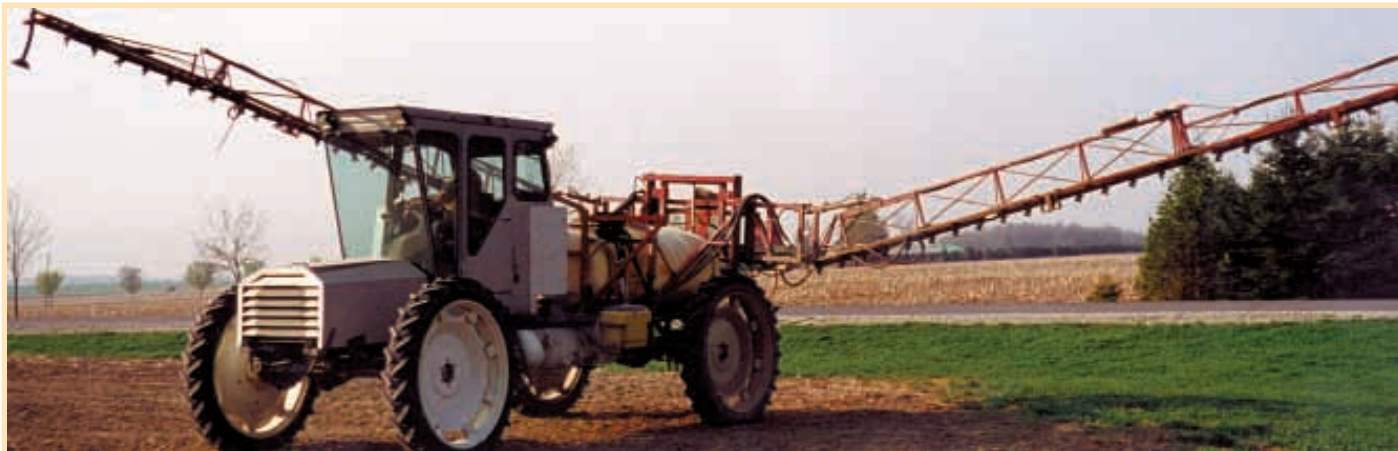
"I built it myself for only about $20,000," says Bob Wood about the self-propelled sprayer he built out of a 1-ton GM 4-WD truck frame. It has a 500-gal. tank and a 60-ft. boom.
