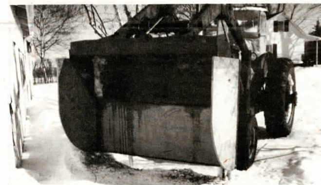
Extension's bolted to the loader so it can be easily removed.
