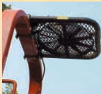
Fan is enclosed in a 2 by 3-ft. steel frame and secured with custom-made brackets.
