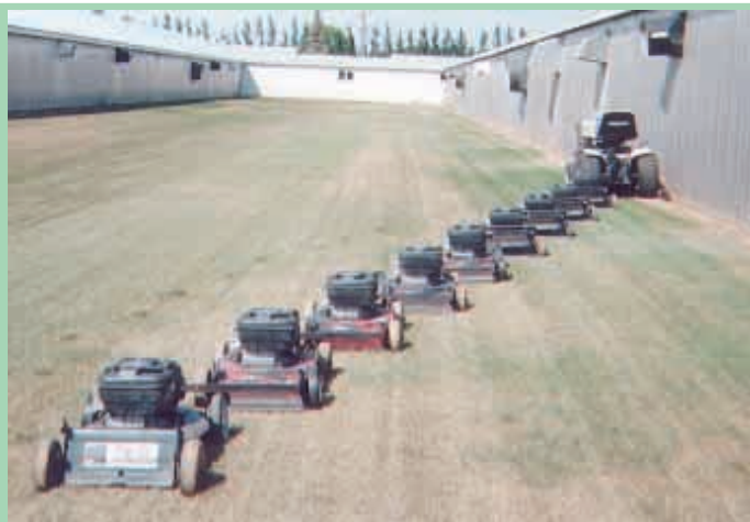
Aron Wiebe put together this mower train that cuts a 15-ft. swath of grass at a time. Wiebe drives an 18 hp riding mower and pulls nine push mowers behind.
