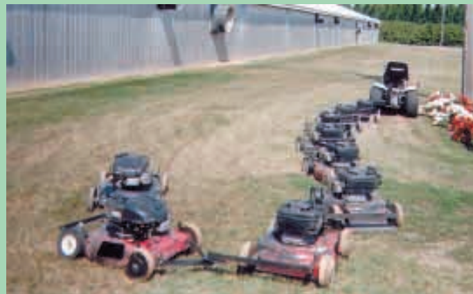
Mower train can make sharp U-turns to snake around trees and poles.
