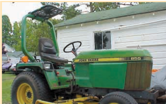
William Russ mounted a downdraft 16-in., 12-volt fan on the rollbar of his riding mower. Fan rotates at 1,700 rpm's, providing plenty of air flow even on hottest days.
