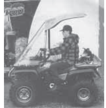
Hardtop ATV cab has gutters that keep rain from running over the side onto driver.
