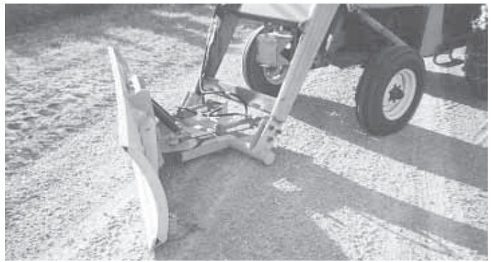
Unique design allows blade to pivot up or down and left or right.
