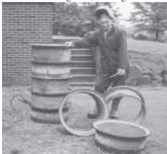
Rims are spot welded every 6 in. around the edges.
