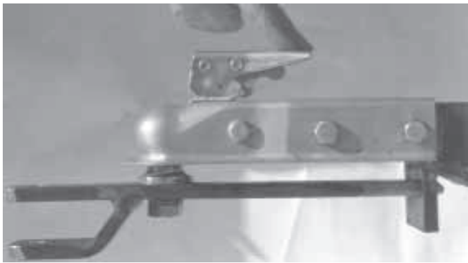
Adaptor lets you switch from ball hitch to pin hitch in seconds.
