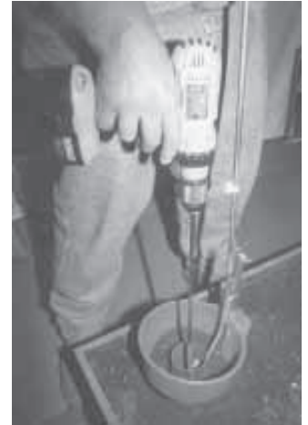
E-Z planter catches the dirt as you dig hole, then puts it back once the seedling is in place.
