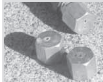
Pipe caps have one or more holes, depending on conditions.
