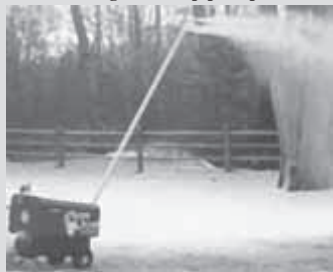
Homemade snowmaker mounts on a stand. Water comes up through bottom pipe and air is injected from one side, forcing water mist out through hole in pipe cap.
