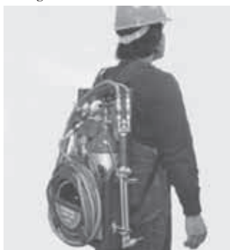
Backpack-carried unit allows user to carry enough gasoline and oxygen for 40 minutes of cutting.
