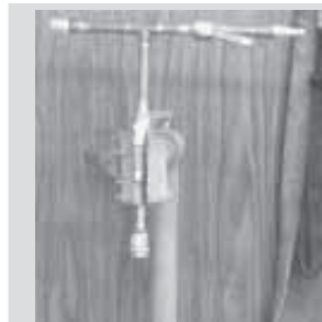
Homemade snowmaker mounts on a stand. Water comes up through bottom pipe and air is injected from one side, forcing water mist out through hole in pipe cap.
