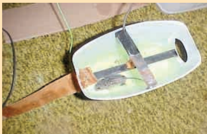
Fence charger can be used to kill mice anywhere, says inventor Keith Lamb. Mouse gets electrocuted as it reaches up to touch bait.
