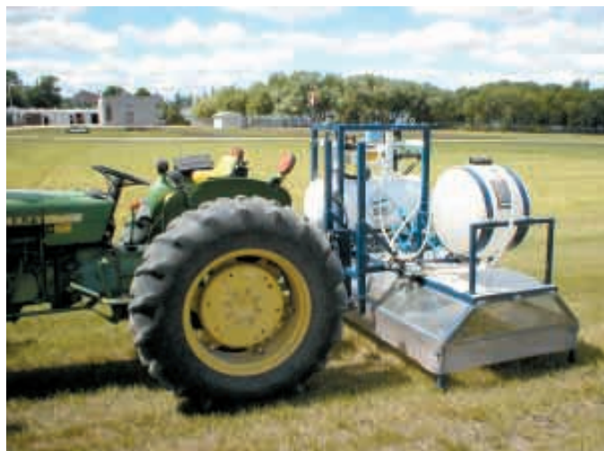
Specially designed, 3-pt. mounted sprayer is equipped with a 6-ft. wide shroud that contains two booms - one to apply ammonia gas and one to apply water.
