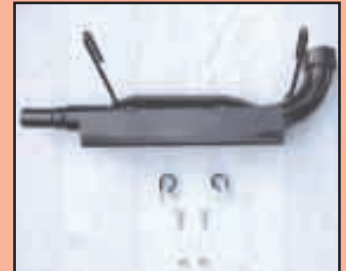
Unit measure 3 1/2 in. sq. by 18 in. long and hangs from ATV's rear rack on two rubber-coated hooks. It slides over end of muffler and is held in place by two bolts.
