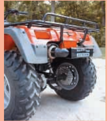
ATV Silencer is designed for hunters and anyone else who wants a quieter ride. It reduces noise level of an ATV by more than half.
