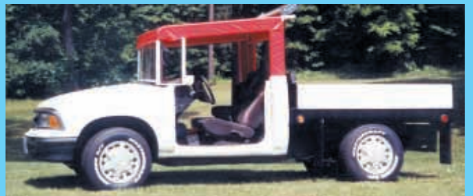
Dale McPeake converted a 1997 GMC Sonoma 4-WD pickup into this utility vehicle that he says works better than commercial-built machines.
