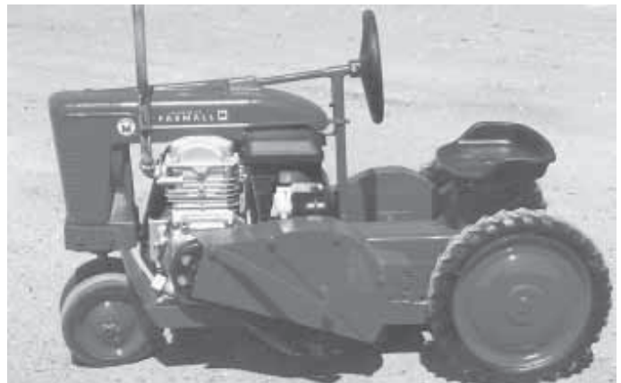
Motorized International Harvester pedal tractor is powered by a 3 1/2 hp Honda gas engine. It direct-drives a centrifugal clutch which chain-drives the rear axle.
