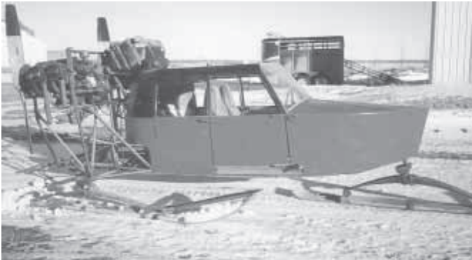
Propeller-powered sleds were popular in the late 1950's and 60's in the Northern Plains. Gleason added a second engine to this early model.
