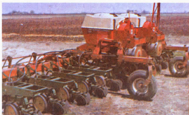
Gangestad's "hybrid" planter features Max-Emerge units, and a Cyclo air delivery hopper.
